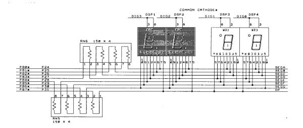
The digit 3, 2, 1, and 0 are driven by PP0, PP1, PP2 and PP3, respectively. The 7-segment LED is turned on one at a time at 250 Hz refresh rate. It's so fast that our eyes will perceive that all 4 digits are turned on at the same time. To display the number 1234 on the 7-segment display, the following steps should be taken:
