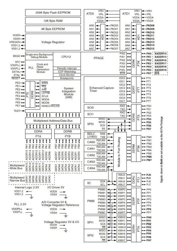
Fig 1-2: MC9S12DG256 MCU block diagram
