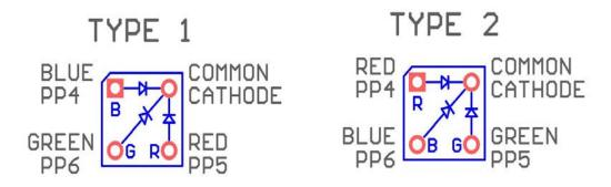
The Common Cathode RGB LED comes in two different pin configurations as shown above. In Type 1 the PP4, PP5 and PP6 control Blue, Red and Green LEDs, respectively.
