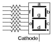
The segment A, B, C, D, E, F, G and Decimal Point are driven by PB0, PB1, PB2, PB3, PB4, PB5, PB5 and PB7, respectively. The hex value of the segment code is shown in the following table:
