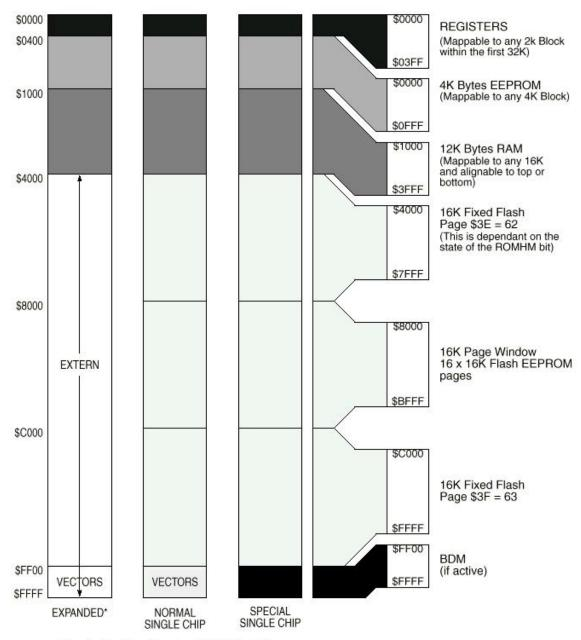
Assuming that a '0' was driven onto port K bit 7 during MCU is reset into normal expanded wide or narrow mode.
